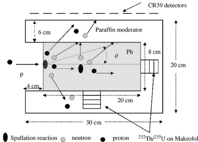
Fig. 1. A cross-section of the experimental setup with a sketch of particle multiplication along the target.
