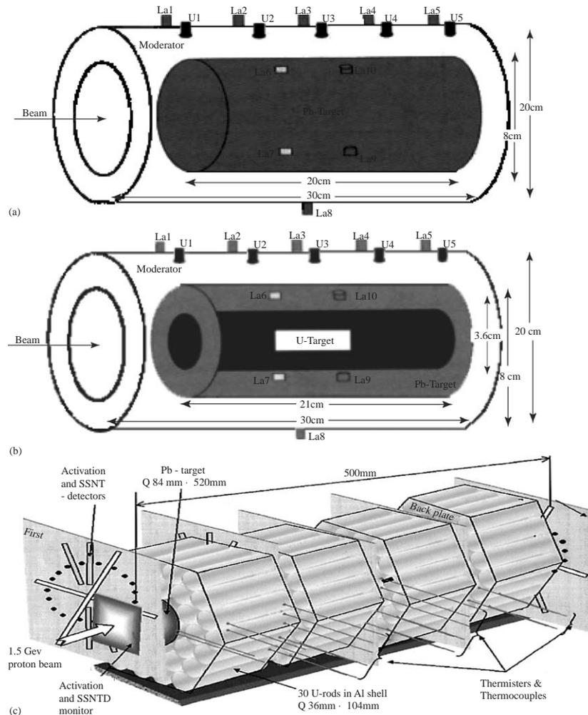
Fig. 1. Different set-ups studied as spallation sources: (a) Pb target with paraffin moderator, (b) Composite natural U and Pb target with paraffin moderator, (c) Pb target enveloped by natural U rods (U blanket).
