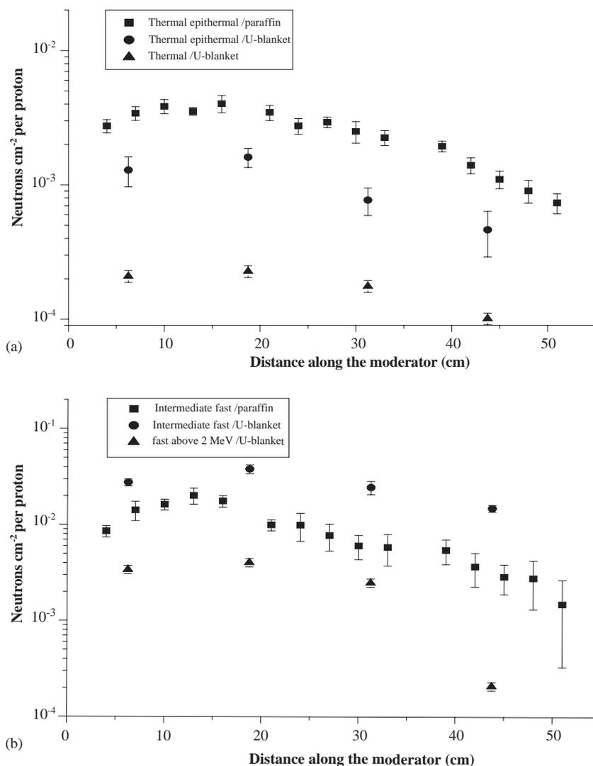
Fig. 2. Spatial neutron distribution along the moderator surface: (a) thermal–epithermal and (b) intermediate–fast neutrons for Pb target and Pb target plus U blanket (50 cm). In (a) thermal neutrons from <sup>235</sup>U fissions and (b) fast neutrons from <sup>232</sup>Th fissions are also seen.
